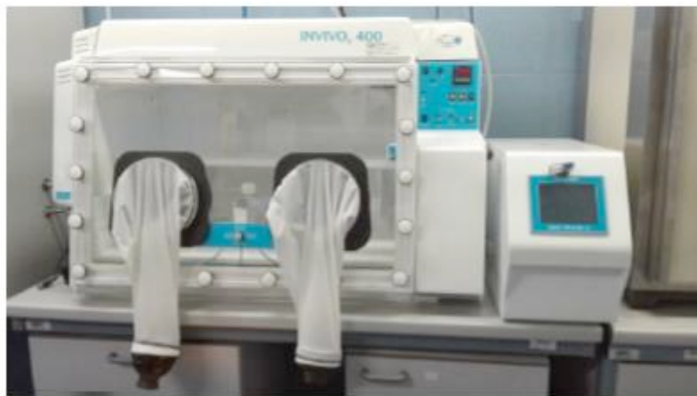
Figure 16: the hypoxic InVivo 400 workstation (Ruskin, Pencoed, UK).
