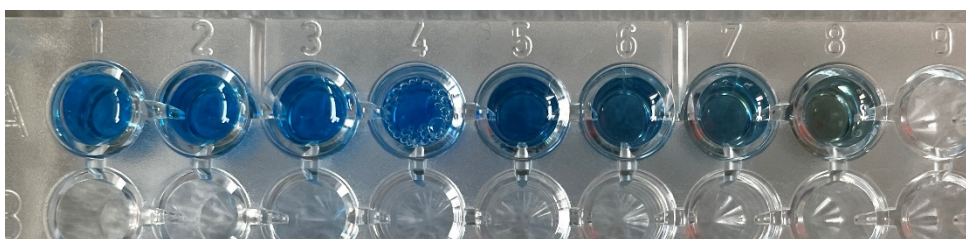
Figure 47: Biorad™ reaction in presence (wells 1-7) and in absence (well 8) of protein.
