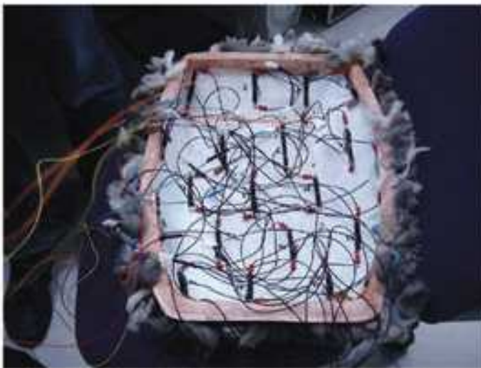
Figure 11. The inner shell of the interactive fur with Nitinol springs.
