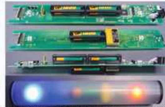
Fig. 5. The PCB seen from the top, the bottom, the side, and an assembled RP
