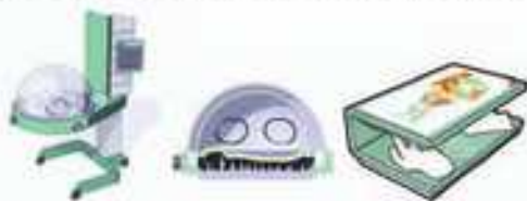
Figure 1: The incubator prototype model, the mattress embedding the moving pins, a map showing pressure points.
