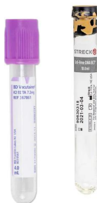
Figure 19: K2 EDTA BD Vacutainer® collection tubes (BD, Franklin Lakes, NJ, USA) on the left, with capacity of 4 ml and plasma preparation must begin \leq 4 hours from time of blood draw. On the right, Cell Free DNA BCT collection tubes® (Streck, La Vista, NE, USA) with capacity of 10 ml; plasma preparation must begin \leq 3 days from time of blood draw.
