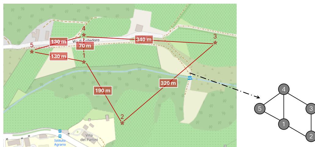
Figure 2. Geographical map of the sensor network deployed in the chosen test site and corresponding graph representation defined according to a spatial proximity relationship (i.e., each node is connected to its two nearest neighbors in terms of straight-line distance).
