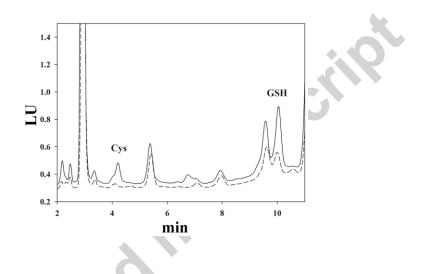
**Fig. 2.** Representative chromatogram obtained from rat liver homogenate derivatized for GSSG analysis. Liver was homogenized and rapidly treated with NEM. GSH was measured on the supernatant after reduction of the disulphide bridge by DTT and thiol labelling with mBrB [67]. GSH eluted at 10.05 min of retention time. A peak corresponding to cysteine (Cys) was also observed at 4.211 min of retention time. The dotted line shows the chromatogram obtained from a blank run.
