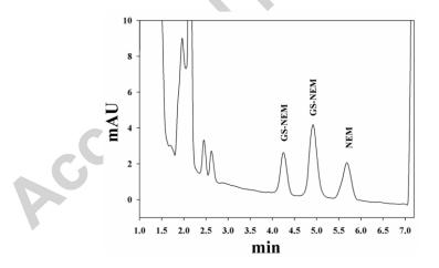
**Fig. 1.** Representative chromatogram obtained from a blood sample derivatized for GSH analysis. Blood from a healthy donor was collected in the presence of NEM. Sample was then deproteinized and supernatant was analysed by reversed-phase HPLC at 265 nm wavelength [61]. The GS-NEM
