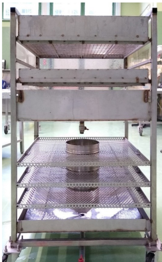
Fig. 40. The multi-sieves tool developed in collaboration with the Department of Comparative Biomedicine and Food Science of the University of Padua and the IZS (Experimental Zooprophyllactic Institute) of Piemonte, Liguria and Valle d'Aosta. Source: Corazzola et al. (2021).
