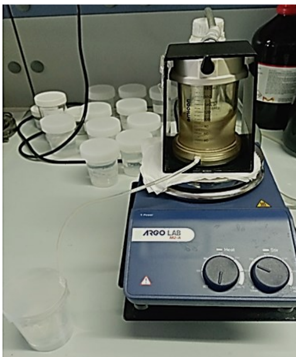
Figure 16. Ultrafiltration equipment connected with collective batch.
