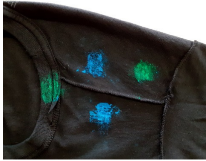
Fig. 3.6 Estimate of the fabric portion involved in the grasp, with and without the electromagnet exploitation (blue and green marks, respectively). A smaller portion produces less wrinkles, increasing the grasp precision.
