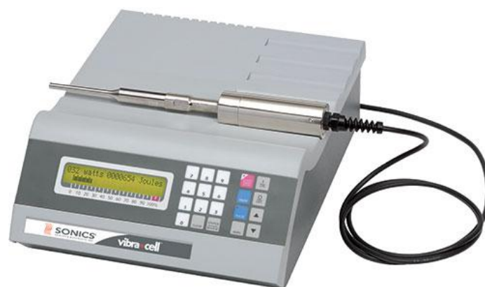
Figure 11: The sonication device employed to homogenize whole platelets
