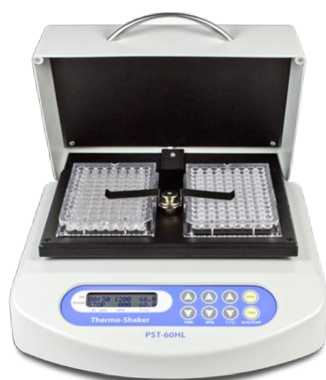
Figure 12: The Thermo-shaker used for all ELISA incubation steps
