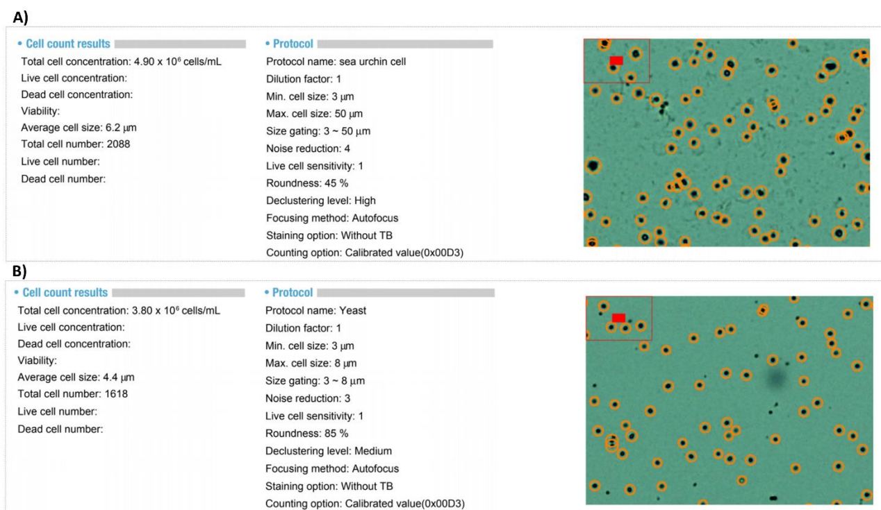
Figure S4.1. Luna II Automated cell counter (Logos Biosystems Inc) instrument settings used for cell counting. Settings for (A) heterogeneous coelomocytes populations (phagocytes, vibratile cells, white and red amebocytes) suspended in CF and (B) yeast cells of Saccharomyces cerevisiae suspended in 0.22- \mu m filtered NSW.
