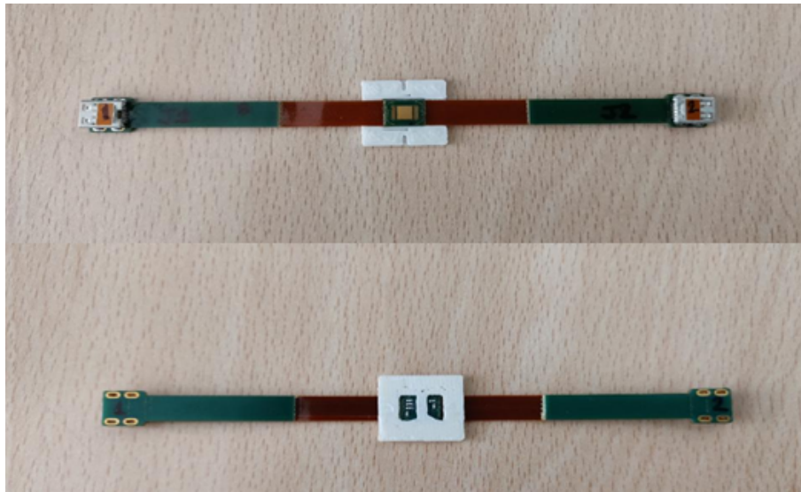
Figure 2.15: The PCB flat cable on which the APiX detector is fixed: front view (top) and rear view (bottom).
