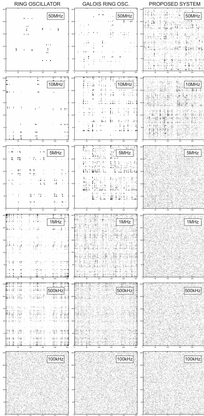
Figure 2.9: Pattern distributions of successive generated bytes on the plane (b_n, b_{n+1}) , for the three considered DNOs, for different sampling frequencies. Each column shows the distributions for a topology, sampled at frequencies going from 100 kHz (lower plots) to 50 MHz (upper plots).
