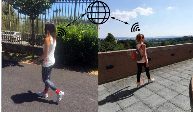
Figure 2.5: The proposed system for remote social walking : i ) the anklet device (1) measures user A 's gait cadence; ii ) the smart-phone (2) receives the stride duration data via Bluetooth; iii ) the information is sent to a server via Internet communication (3); iv ) the server sends the update to user B 's smart-phone; v ) the smart-phone (2) commands vibrations at the user's anklets (1).
