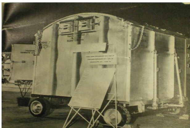
Fig. 2 Container refrigerants for carriage of perishable foodstuffs.
