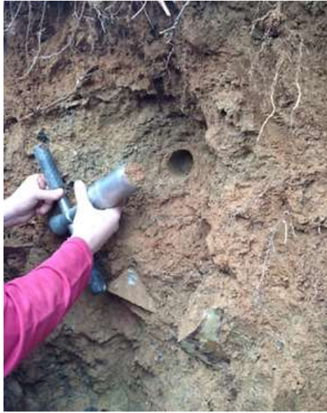
Figure 2-13 The collection of undisturbed samples for unit weight determination
