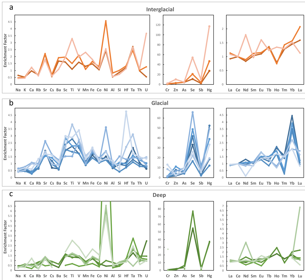
Figure 4.8: Enrichment Factors calculated for INAA measurements. Samples were divided into 3 categories: interglacial samples (a), glacial samples (b) and deep samples (c). Each line represents a single sample. For deep samples, some elements (Ba, Zn, Se, Hg, Ho, Tm) were not considered in all the samples, leading to some broken lines.
