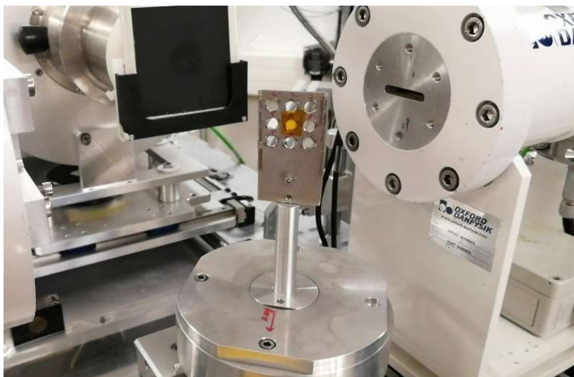
Figure B11. Sample holder with mounted sample, stucked between Kapton tape (yellow). A plastic glove transparent to X-rays continuously fluxed with argon (not shown in the figure) was put over the sample holder during data acquisition.
