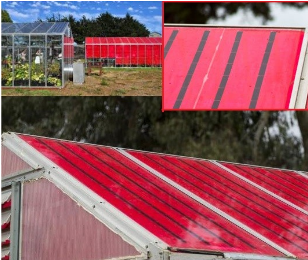
Fig. 30: Greenhouse covered by LSC and the control (on the left, up) and some details of roof. In California, the first LSC greenhouse, LR305 based, was tested controlling efficiency, energy production and plants growth over its for one whole year 128 .
