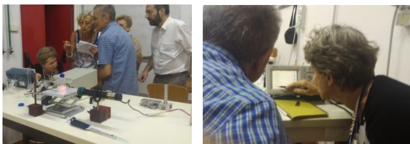
Figure 6. The experimental set-up for the reaction between sodium thiosulphate and hydrochloric acid (on the left) and teachers that analyse the data on the oscilloscope in order to determine the characteristic time of the reaction.
