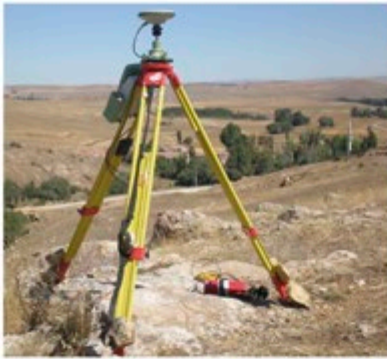
1 – Differential GPS survey: Static modality (left) and Real Time Kinematic (right).
