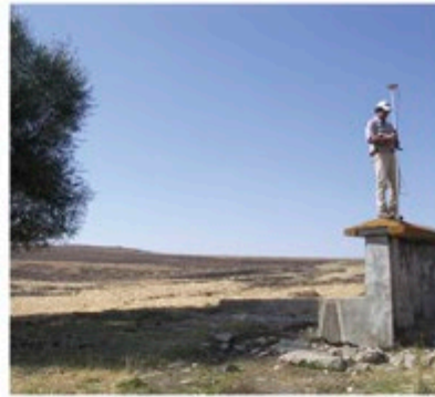
1 – Differential GPS survey: Static modality (left) and Real Time Kinematic (right).
