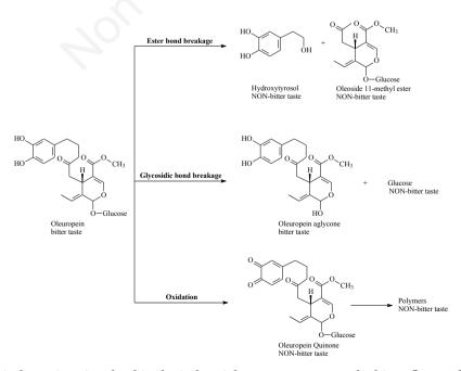
Figure 6. Main chemical reactions involved in the industrial process to remove the bitter flavour from olives.
