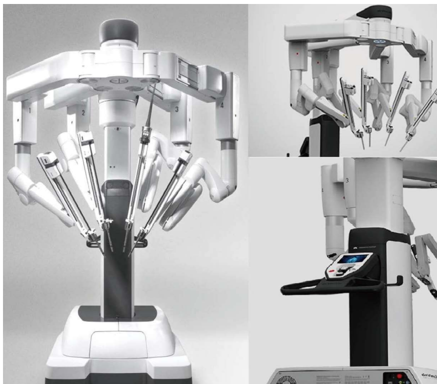
Figure 1 New-generation da Vinci Xi™; the system is more versatile and better manoeuvrable, the robotic arms are thinner and arranged in a more ergonomic way, enabling multi-quadrant procedures without repositioning the system.
