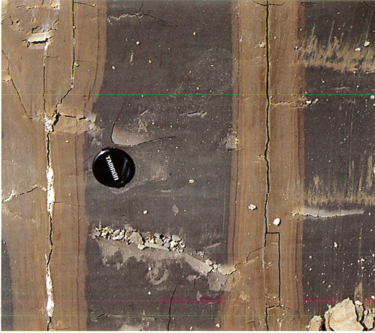
Photo 3 - Two parallel joints from a quarry plane with «varved» salbands. The one of the left shows discontinuous chalk filling; the joint opening is due to pressure release caused by quarrying.
