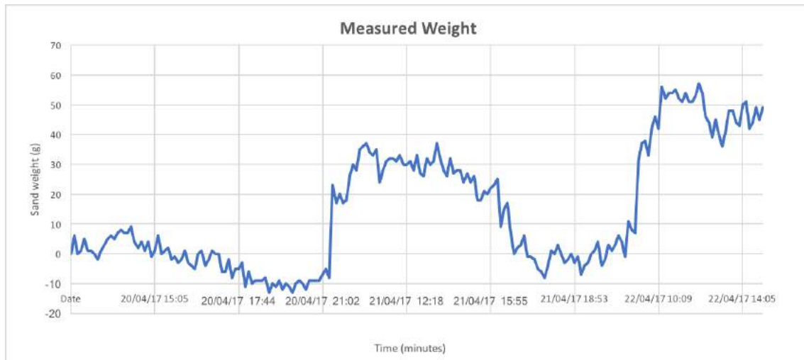
Figure 10. Collected sand weight during the data acquisition campaign carried out on the beach of Marina di Tirrenia.
