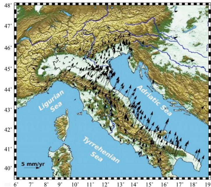
Figure 2. Residual horizontal velocities (black vectors) of the GPS sites with respect to a fixed Eurasian frame (Euler pole at 54.23°N, 98.83°W, \omega = 0.257^\circ/\text{My} , [37]). Data and methodology described by [34] [35].
