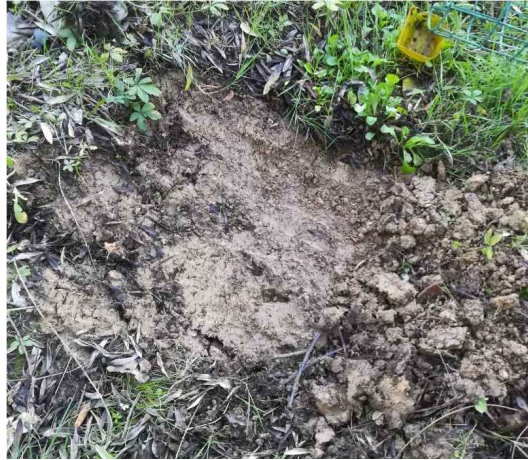
Figure 4.7: Compacted soil surface after node burial for the test assessing the impact of soil compaction on RSSIs.
