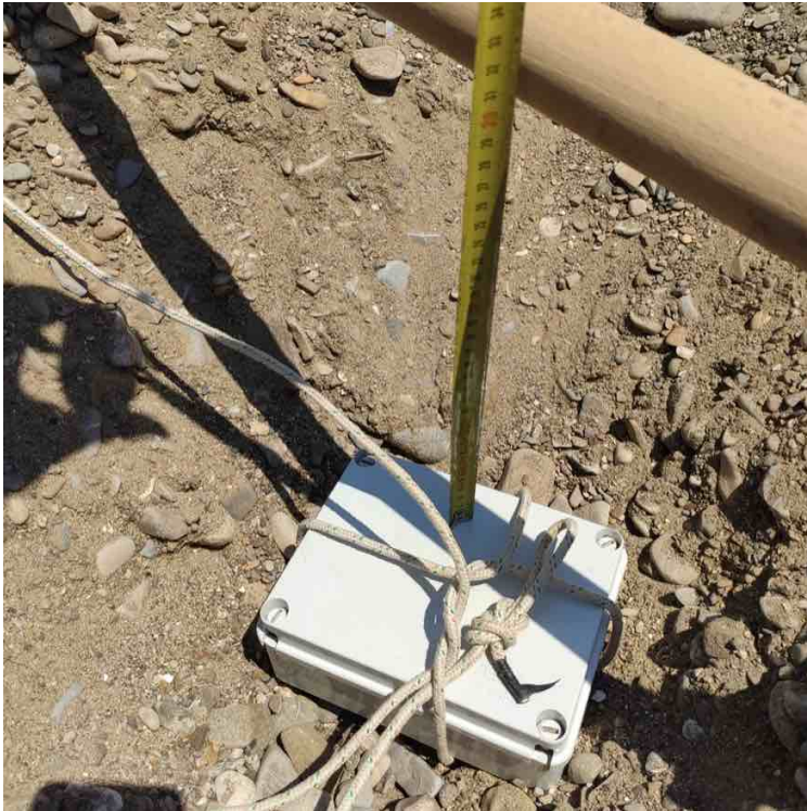
Figure 4.8: The IoUT sensor node during the field measurement campaign. Ropes were used to ease the node retrieval.
