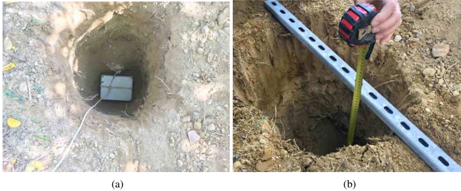
Figure 4.3: The LoRaWAN IoUT sensor node 50 cm underground during the preliminary laboratory measurement campaign for LoRaWAN links.
