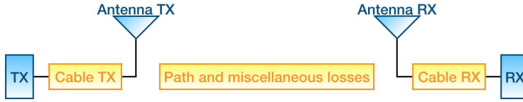
Figure 3.1: Gains, in blue, and losses, in yellow, of a communication channel to be accounted within link budget equation.
