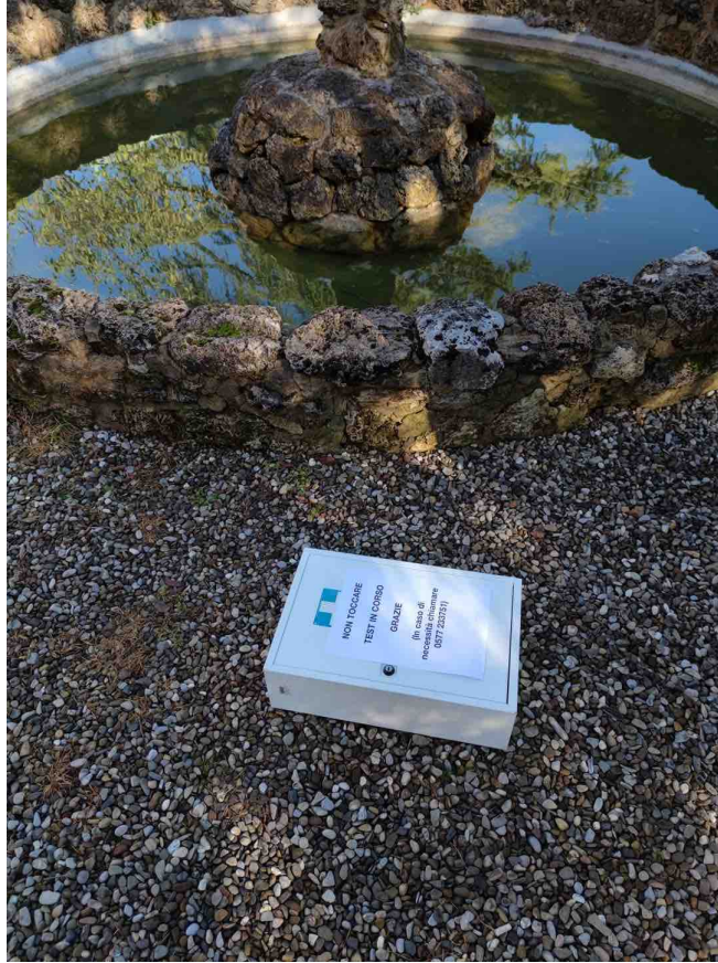
Figure 6.4: Test setup for the through-metal links exploiting LoRaWAN and NB-IoT technologies.
