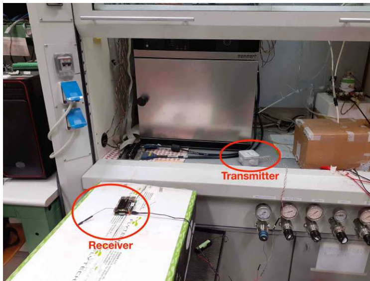
Figure 7.3: Gas exposure test setup showing the transmitter within the containment box and the gateway in front of the fume extraction plant.
