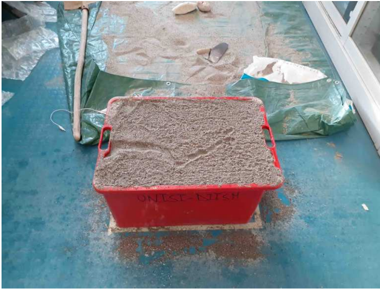
Figure 8.14: Plastic case with sand that was exploited for laboratory tests on the effect of VWC on LoRaWAN UG2AG links.
