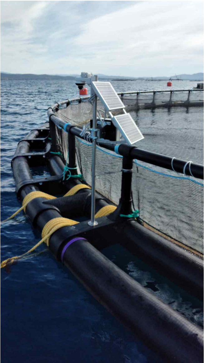
Figure 8.10: VSU prototype offshore installed on a cage floating structure.
