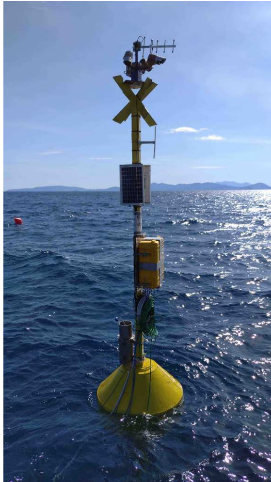
Figure 8.1: Seamount buoy on which the sensor node was installed.
