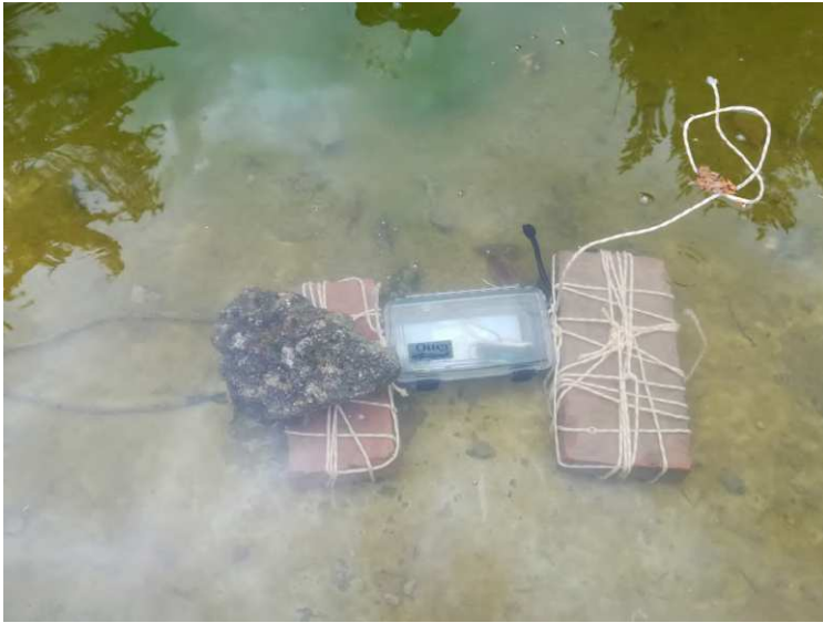
Figure 5.2: Test setup for the UW2AW links exploiting LoRaWAN and NB-IoT technologies.
