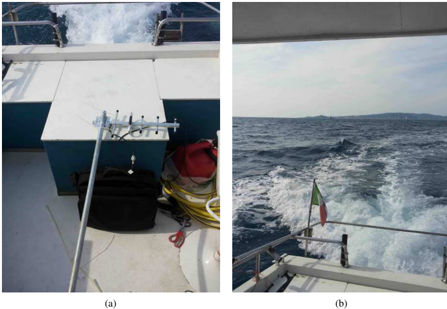
Figure 3.6: Offshore setup for the short-term measurement campaigns: (a) offshore end node antenna and its pole; (b) view approaching the tests spot.
