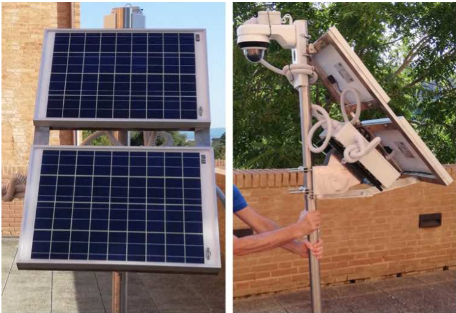
Figure 8.9: Realisation of the VSU: photovoltaic panels (left) and pole with camera and IP56 box containing the electronics (right).
