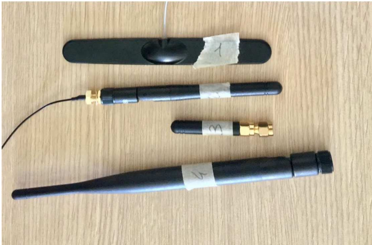
Figure 4.2: Employed antennas during the tests for antenna selection for the LoRaWAN IoUT sensor node. From top to bottom: A_1 , A_2 , A_3 and A_4 .
