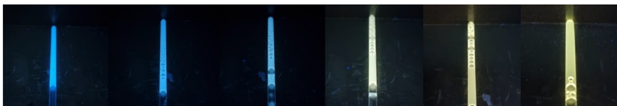
Figure 5. Comparison of the fluorescence emission of the reaction mixtures obtained with HSA (67 mg, 1.0 micromol) in D 2 O (1.4 mL) containing PBS (Aldrich) at pH 7.4 and compound 7 (0.48 mg, 1.0 micromol), which was added as a (50 mM) solution in DMSO- d 6 (0.020 mL). The reaction mixtures contained into a 5 mm NMR tube were heated at 50 °C and were photographed at regular time intervals (0, 1, 2, 4, 8, and 24 h, from left to right in the sequence) under excitation at 365 nm.
