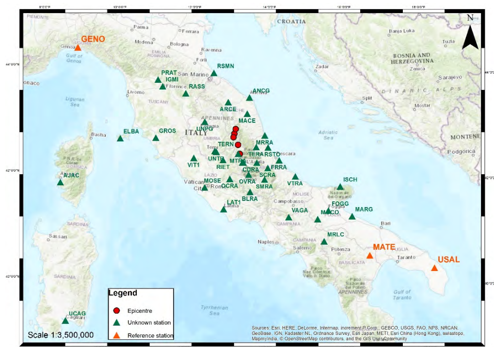
Figure 4. Location of the GNSS permanent stations processed within Bernese software: the different triangles represent some reference stations (others, most of them, fall outside this map) and the position of stations to be calculated; dots stand for the epicenter position of the major seismic events (as reported in Table 1).
