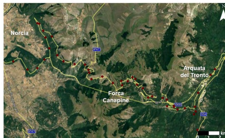
Figure 15. Example of geometric leveling lines characterized by the presence of hairpin bends that adversely affect the calculation of benchmarks position (rhombus). The lines represent the provincial (SP) and state (SS) roads (background image from Google Earth image, earth.google.com/web/ accessed on 9 February 2022).
