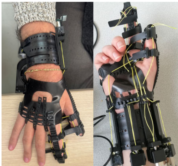
Figure 1. The glove with the thumb and index modules worn by two users.
