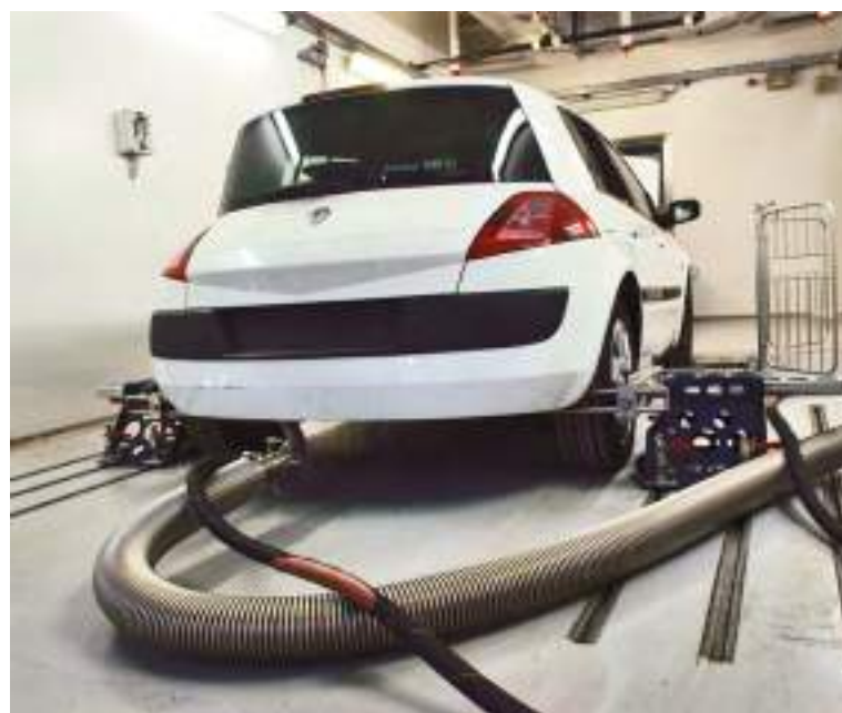
Execution of exhaust gas measurements in the VELA laboratory.
