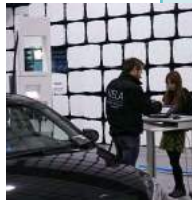
VeLA 9: an e-mobility electromagnetic testing facility.
