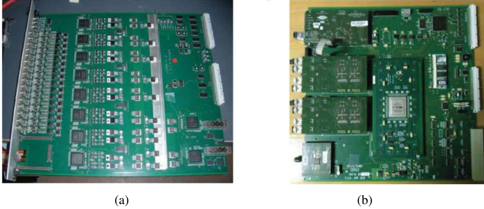
Figure 69. Photographs of the LUCID 2 readout cards: (a) LUCROD and (b) LUMAT.
