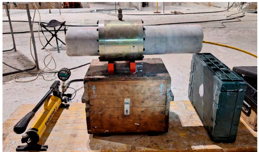
Figure 8. Stages of biaxial compression testing using the Hooke biaxial cell at the Ravalunga quarry.
