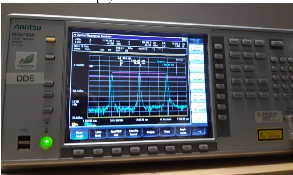
Figure 3.7: The three reflected spectrums centred in the chosen wavelengths, related to the three FBGs elements.
