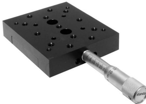
Figure 3.2: Stable steel translation stage (called Stage 1) 7T67-25 by 'standa' company.
