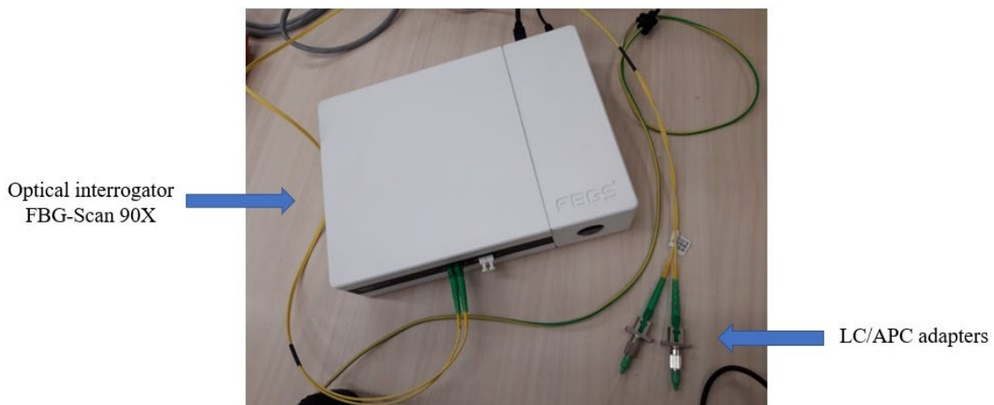
Figure 3.7: Optical interrogator FBG-Scan 90X and optical fibers connectors.
