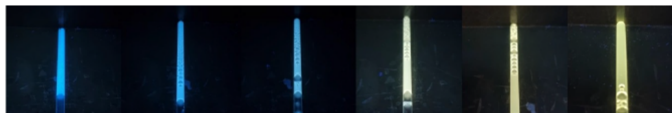
Figure 5. Comparison of the fluorescence emission of the reaction mixtures obtained with HSA (67 mg, 1.0 micromol) in D 2 O (1.4 mL) containing PBS (Aldrich) at pH 7.4 and compound 7 (0.48 mg, 1.0 micromol), which was added as a (50 mM) solution in DMSO- d 6 (0.020 mL). The reaction mixtures contained into a 5 mm NMR tube were heated at 50 °C and were photographed at regular time intervals (0, 1, 2, 4, 8, and 24 h, from left to right in the sequence) under excitation at 365 nm.
