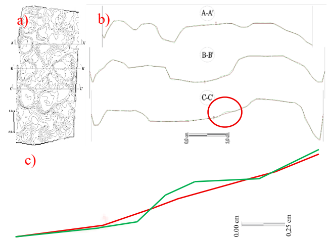
Figures 6 a-b-c: contour plot of block no. 14 (a) and roughness profiles (A-A'; B-B'; C-C') (b); in green the profiles derived from digital sectioning; in red those derived from the profilometer; (c) detail circled in red of the C-C' profile.
