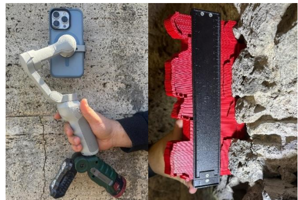
Figures 3 a-b: a) Gear setup: Apple iPhone Pro on 3-axis gimbal and LED light; b) acquisition of roughness profiles using the comb profiler
