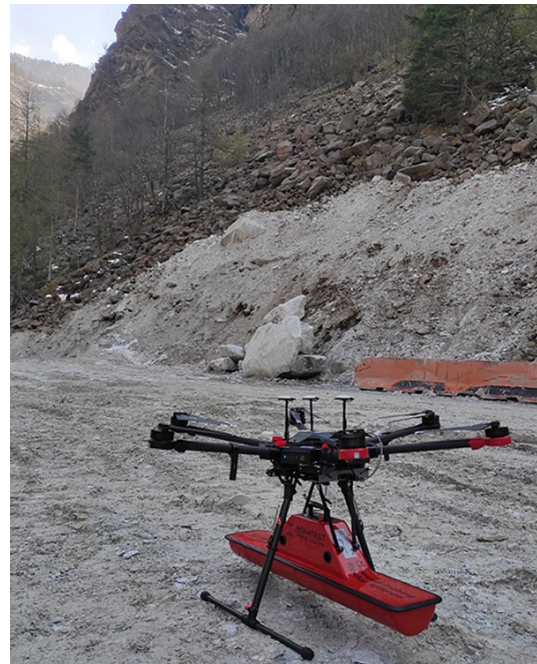
Fig. 4 COBRA Plug-in GPR Model SE-150 and DJI ® Matrice 600Pro drone.
