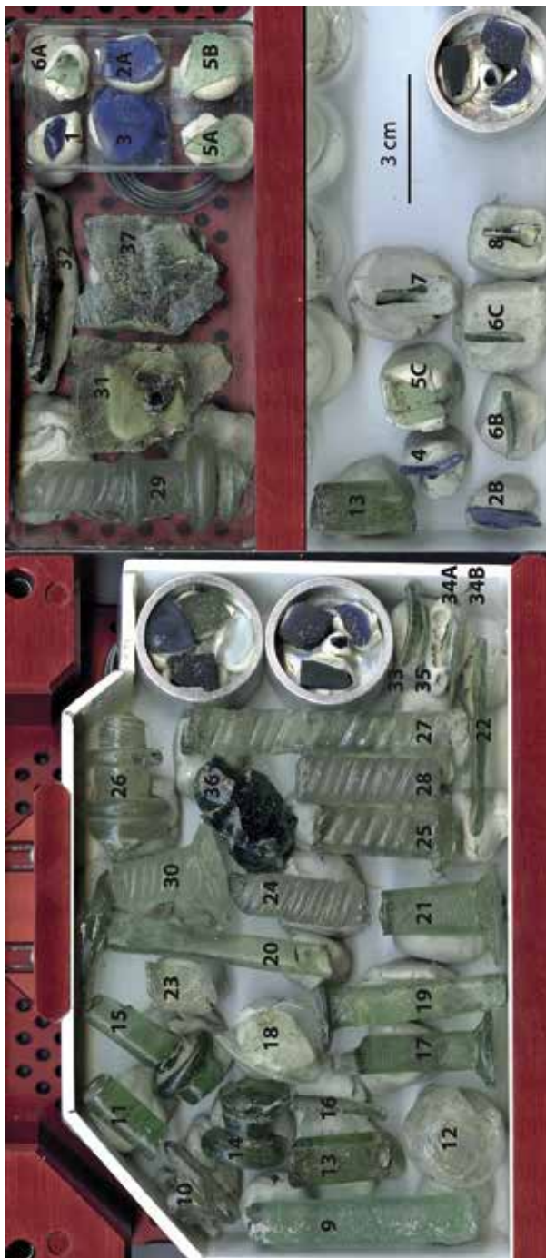
Fig. 2. LA-ICP-MS analytical cell (S155 from Resonetics) used for the analyses of the Vetricella glass corpus. Samples in the metallic cylinders are the glass standards.
