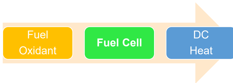
Figure 2.10: Schematic representation of a fuel cell.
