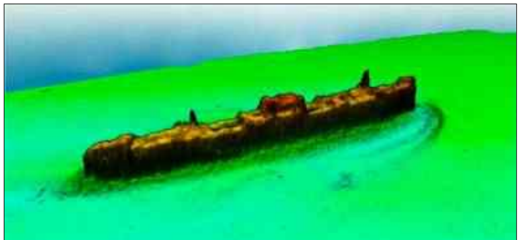
Figure 6. MBES survey of the Tilden wreck (courtesy of ISPRA, Astrea ).
