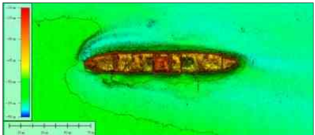
Figure 15. MBES survey of the Tilden wreck and bathymetry (courtesy of ISPRA, Astrea ).
