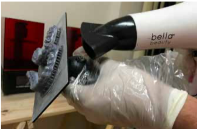
Figure 17. Use of a hair dryer in heated mode to facilitate the removal of resin models from the printing platform.
