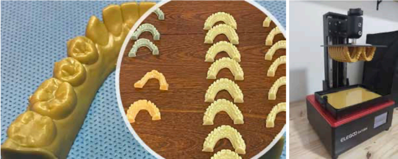
Figure 2. Models printed with 405 nm photosensitive resin at high resolution.
