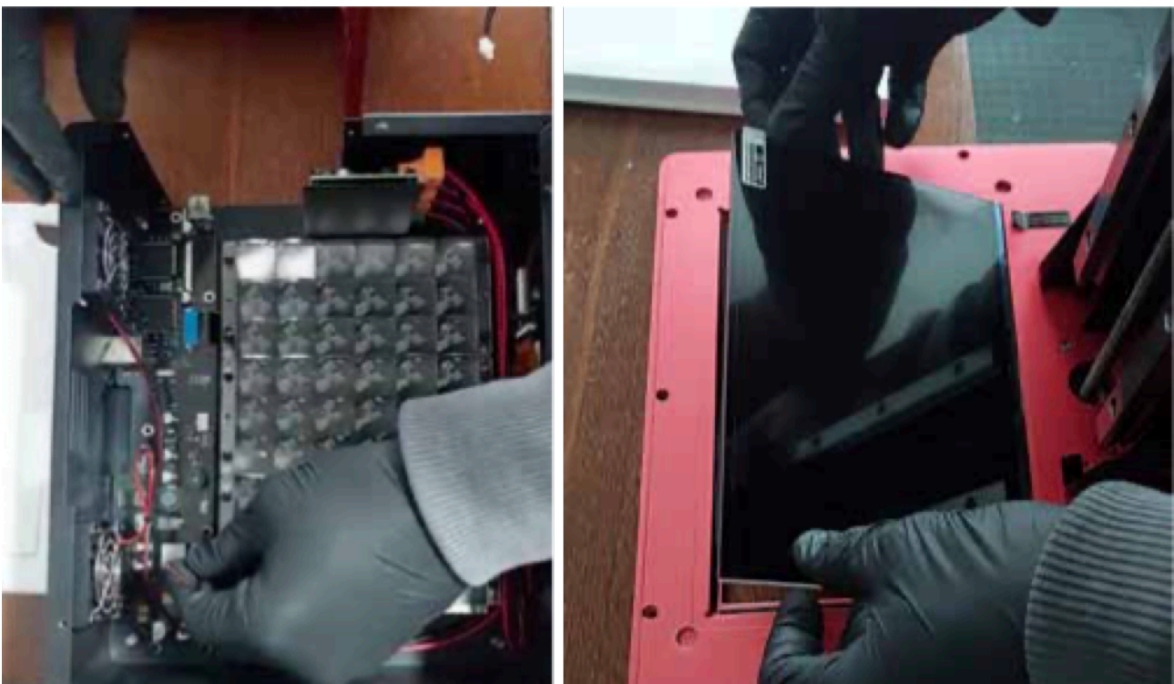
Figure 7 (A-B). M MSLA/LCD printer maintenance: A) Motherboard replacement. B) LCD replacement.
