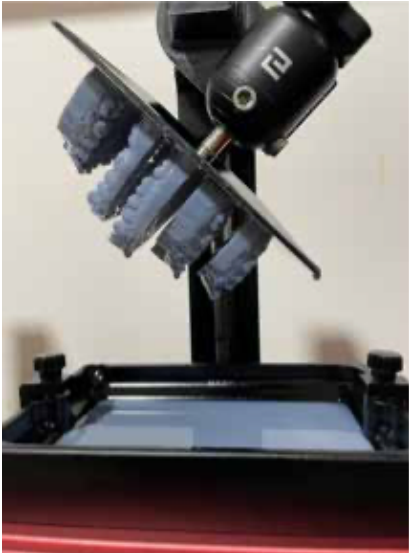
Figure 15. Draining excess resin after printing.
