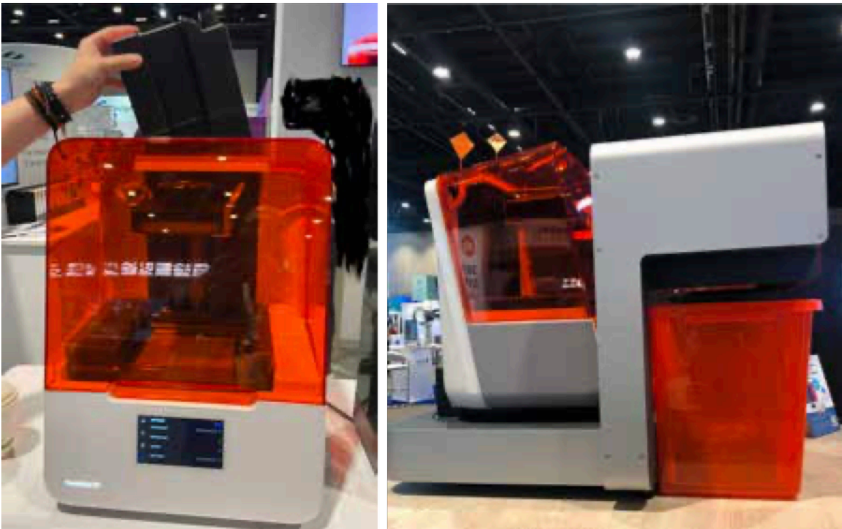
Figure 5 (A-B). Orthodontic 3D printer Formlabs 4P : A) Sealed resin cartridge. B) Automation of the printing process and unloading of already printed models.
