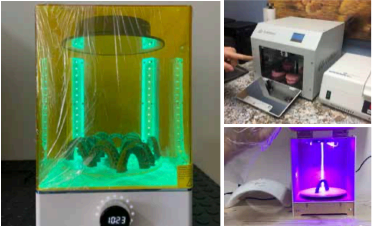
Figure 18 (A-C). UV light post-processing: A) Professional rotary light chamber. B) Professional mirrored light chamber. C) Low-cost amateur UV light chamber.
