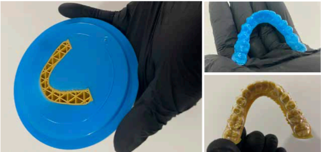
Figure 19 (A-C). Fabricating the aligner: A) Laminate immediately after thermoforming. B) After initial trimming. C) After final trimming and finishing.
