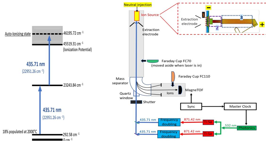
**Figure 1.** Photo-ionization scheme of samarium. Transition wavelengths are given for vacuum.
