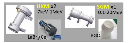
FIGURE 2.3: The HXM and the SGM sensors of the CGBM.
