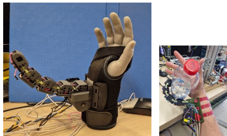
Figure 12. Robotic finger used for the tests.
