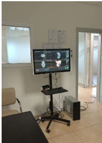
(b) The test room for touchscreen modality: touchscreen display placed on the support with height regulation; workstation with tested software installed, connected through an HDMI cable to an external display; smartphone, placed on support with angular regulation.
