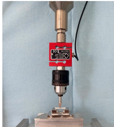
Figure 3. Universal machine for three-point bending test.
