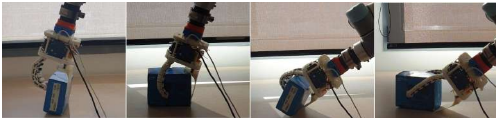
Figure 4.10: Grasps of the cuboids. From left to right: Str. A approaching along the object x -axis; Str. A approaching along the object y -axis; Str. B approaching along the object x -axis; Str. B approaching along the object y -axis;
