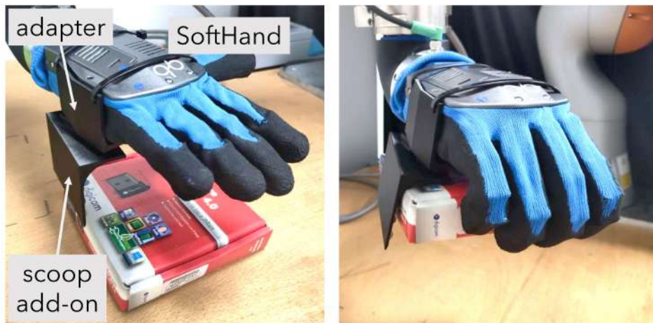
Figure 6.1: Adding a scoop-shaped add-on to a soft hand: pre-grasp configuration, and final grasp. The object cannot be grasped from the top without the scoop, as it is too large. The positioning and geometrical features of the scoop are the result of an automated design approach.
