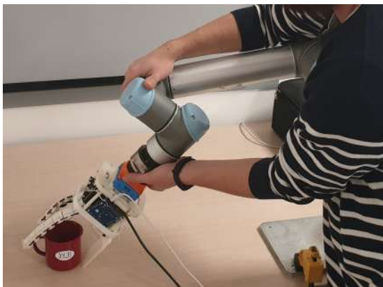
Figure 4.1: Example of human demonstration. A user handles the robot to grasp an object during the training phase.
