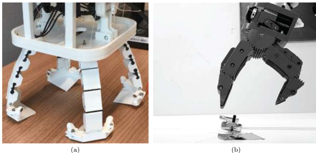
Figure 2.2: Soft hands integrating embedded constraints. a) Quad-Spatula Gripper [5]. b) gripper proposed by Babin [6].
