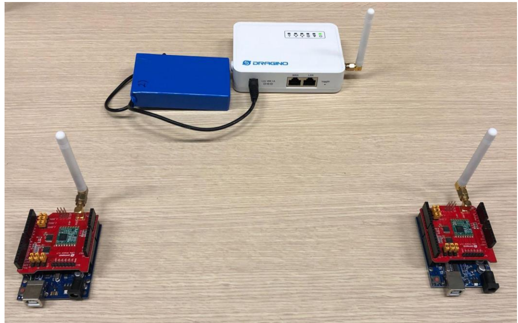
Figure 20. Hardware for laboratory setup with two sensor nodes and a GW (LoRa antennas have been removed when testing the opportunistic protocol in the laboratory to reduce the coverage range).
