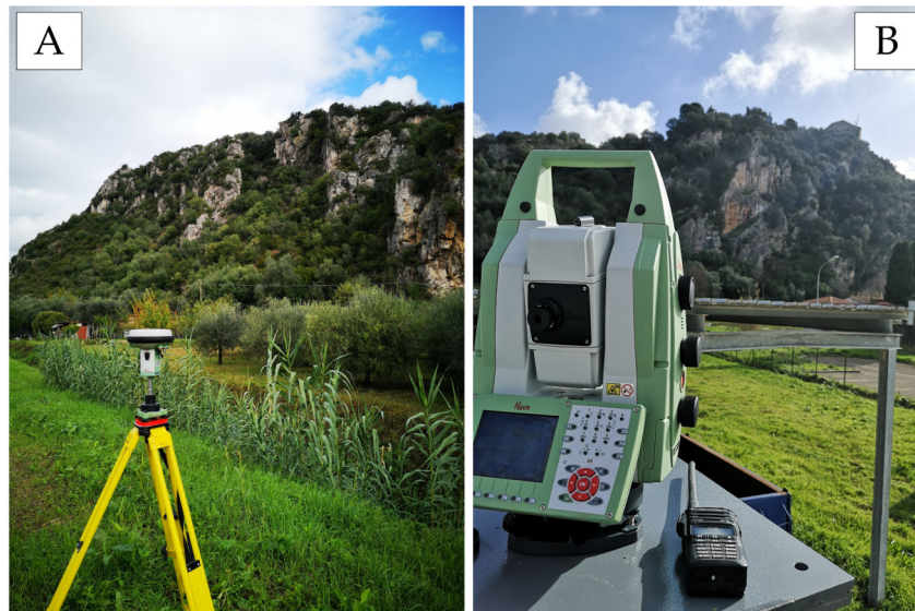
Figure 3.50: Stages of the GNSS (A) and RTS surveys (B).
