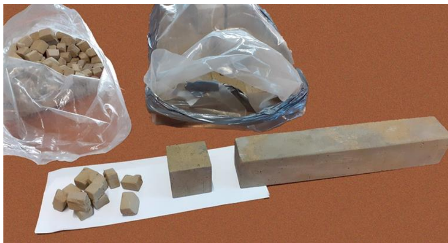
Figure 5.5. Cubic and elongated samples of CFM2 for flexural and compressive strength determinations.
